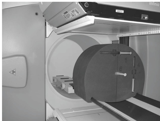
Fig. 2 — To ensure that the CT and SPECT images are correctly co-registered in three dimensions, a series of 6 syringes (3 of which can be seen in the photograph, the other 3 are on the reverse side of the phantom) containing an appropriate radionuclide are inserted into a foam calibration phantom so that they are orientated in three orthogonal planes. When imaged on both the SPECT and CT systems, they permit accurate alignment of the CT and SPECT data. The calibration system is used for the GE Hawkeye 4 system.
