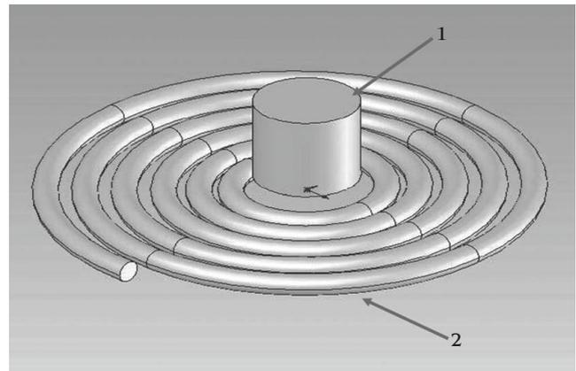
**Fig. 1 — Diagram of electromagnetic vibration actuator composed of a permanent magnet (1) and planar coils (2).**
