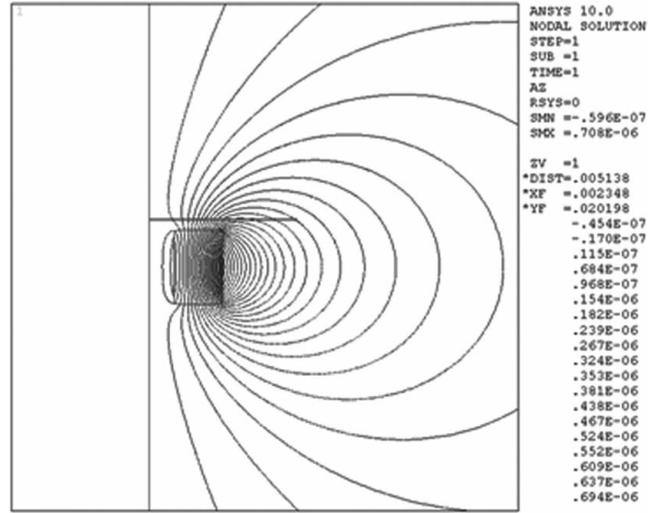
**Fig. 4** — Electromagnetic driving parts: simulation results of magnetic flux distribution of the permanent magnet.
