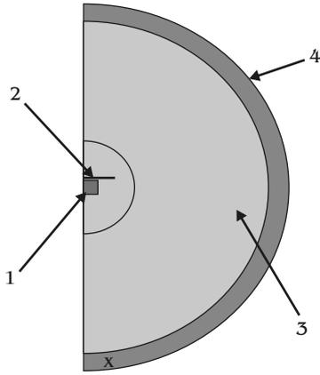
**Fig. 2** — Diagram of an electromagnetic vibration actuator composed of a magnet (1) and planar coils (2). The air (3) and infinite boundaries (4) were also created using computed-aided design.
