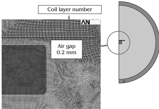
**Fig. 3** — Finite element meshes and the electromagnetic driving parts: schematic diagram of the designed vibration actuator including the magnet, different layers of coils and 0.2mm air gap.
