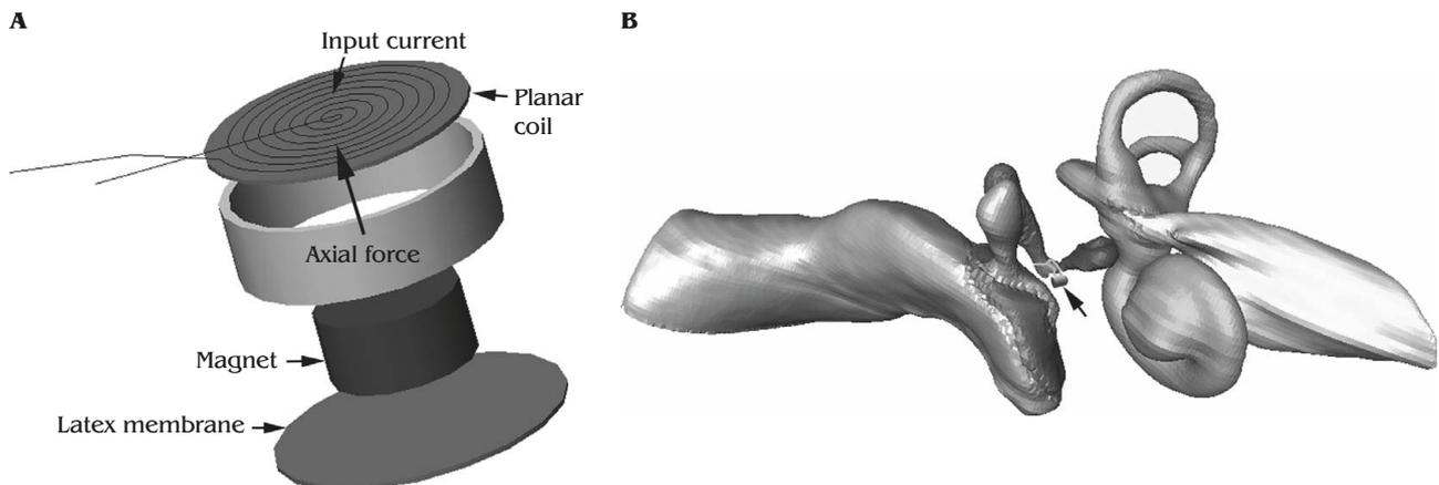
**Fig. 6 — (A) Diagram of the electromagnetic vibration actuator composed of a permanent magnet and planar coils. (B) The new actuator could be attached to the incus by a clip or wire (arrow).**
