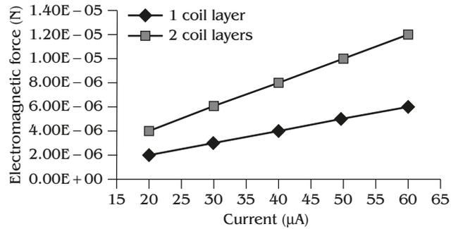
**Fig. 5** — Simulation results of vibration force versus input current at the variance of turns of the coil and at the condition of 0.2mm air gap with various input currents and different number of coil layers.
